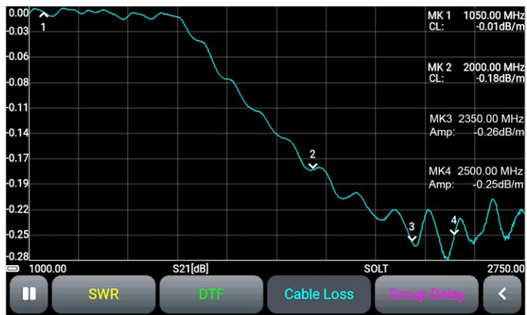
Figure 10.13 - Plot of cable loss measurements
