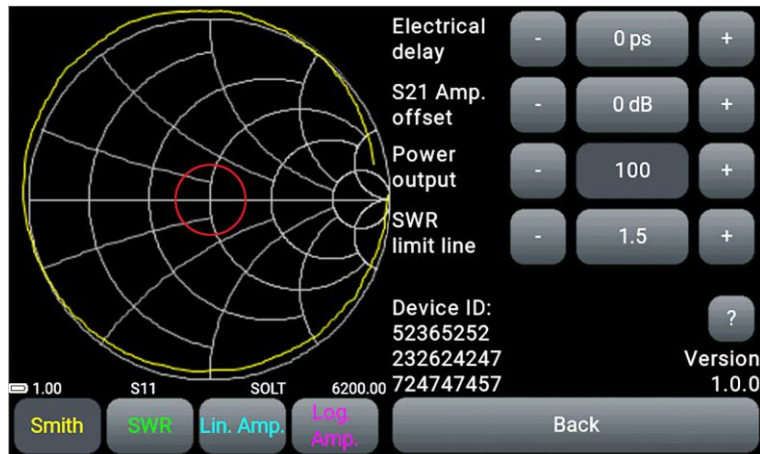
Figure 9.12 - Offset of the calibration plane by an additional cable
