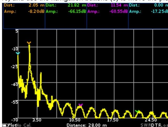
Figure 10.9 – Plot of distance measurement to cable fault
