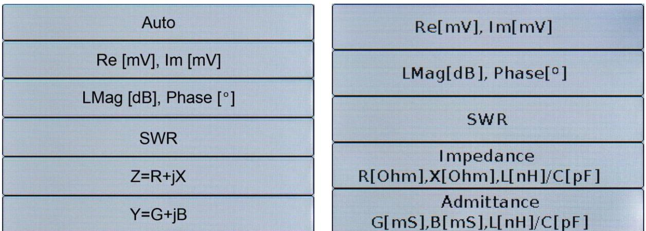
Figure 9.9 – Selecting the type of values displayed by the marker ARINST VR 1-6200 and ARINST VR 23-6200
