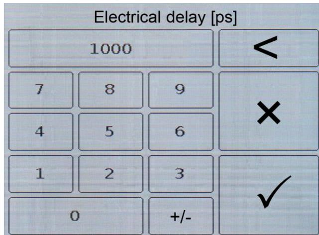
Figure 9.25 – Entering numeric value compensation electric cable length
