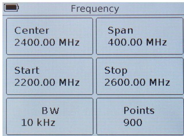
Figure 9.2 – Menu for setting scan parameters
