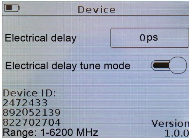
Figure 9.24 – Enabling Electrical delay tune mode
