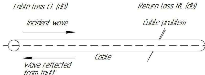
Figure 10.13 – Measurement scheme
