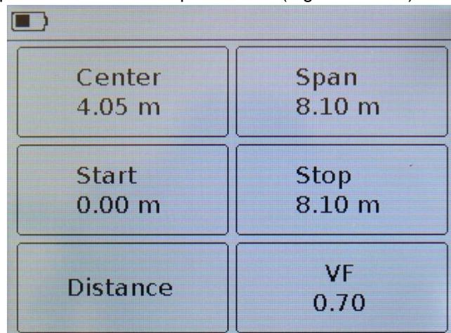
Figure 10.11.2 – Menu for setting the distance scale
