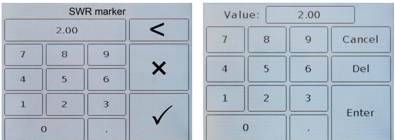
Figure 9.21 – Entering the numerical value of the displayed SWR limit line
