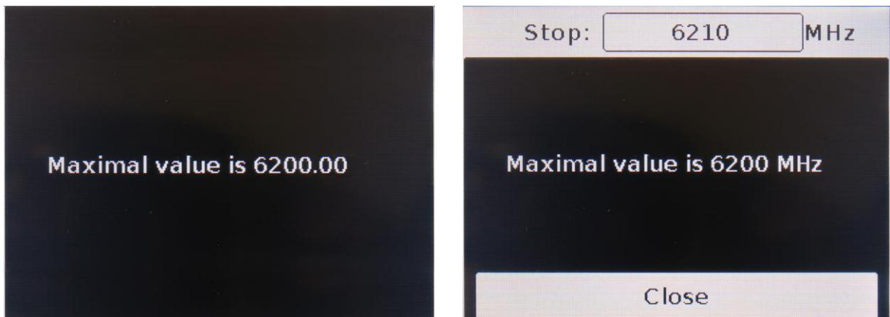
Figure 9.4 – Warning about exceeding the operating range of ARINST VR 1-6200 and ARINST VR 23-6200
