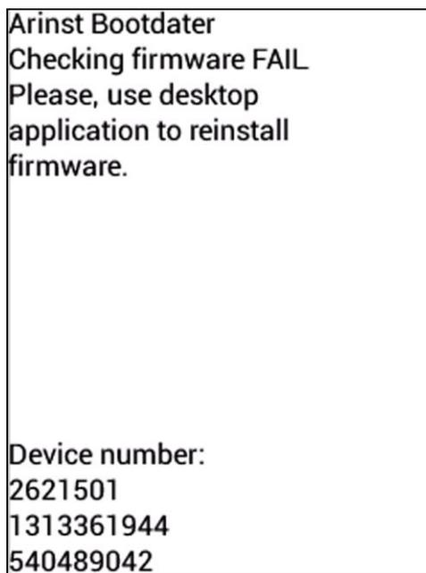
Figure A3.2 – The device screen when the firmware is unsuccessful
